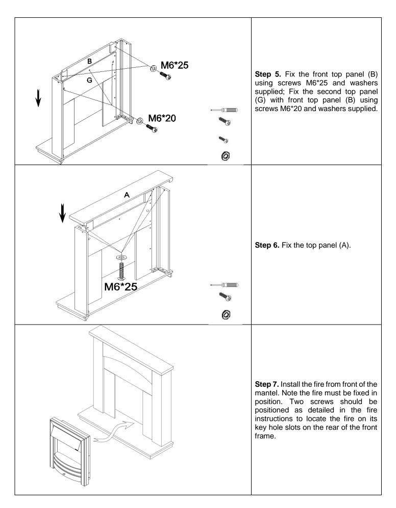
NOTE: This fireplace must be fixed to the wall. Mirror plates are supplied but any other suitable concealed fixing may be used.
